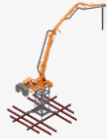
Tower Base Anchored to Deck (Anchored)
