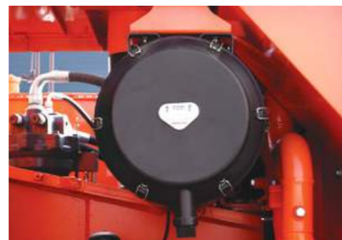
Air filter with pre-filtered dust separator The large capacity forced air cleaner removes over 99% of airborne particles. This reduces the risk of engine contamination and makes cleaning and cartridge change intervals greater. The pre-cleaning system uses centrifugal force to eliminate dust.
